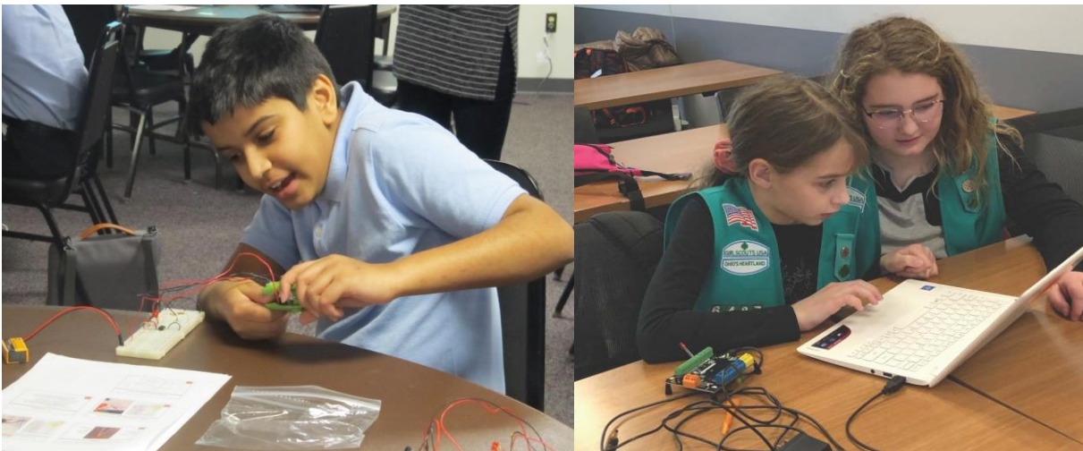
Figure 1. Left: A sixth grader at St Andrew School in Upper Arlington tests the heart rate monitor he just built. There is an IR LED in the potato-chip clip measuring the hemoglobin in his finger. The circuit blinks an LED with his pulse.
